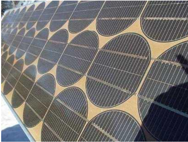
Figure 1 Early example of monocrystalline cells in a module Source: Green Building Advisor (2018)
