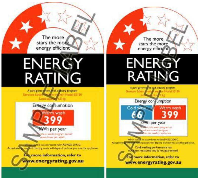
Figure 1-6 Australia’s Energy Rating Label for washing machines. Left: warm wash only; right: warm and cold wash; source (Australian, State and Territory and New Zealand Governments 2014c)
