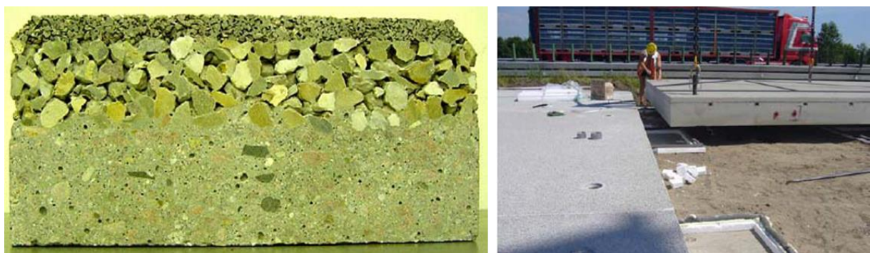
Figure A 17: Example of a novel and multi-layer prefabricated cement concrete pavement for noise reduction (Sandberg, 2009).
