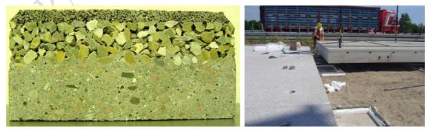
Figure A 17: Example of a novel and multi-layer prefabricated cement concrete pavement for noise reduction (Sandberg, 2009)
