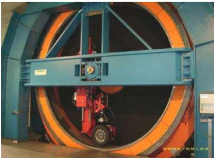
**Figure 3.17: Laboratory drum – Tyre/pavement interaction test facility at BAST, Germany (picture from Sandberg, 2011).**
