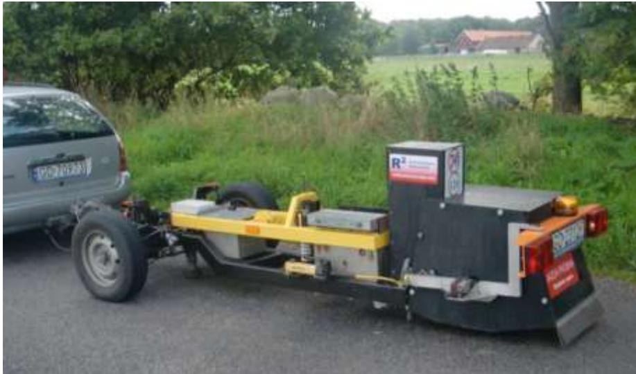
**Figure 3.14: Trailer method – equipment from The Technical University of Gdansk (picture from Sandberg, 2011).**
