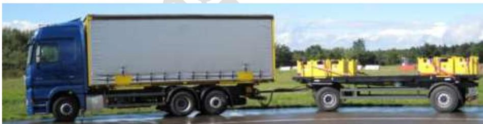
**Figure 3.15: Trailer method – equipment from IPW, Germany (picture from Sandberg, 2011).**
