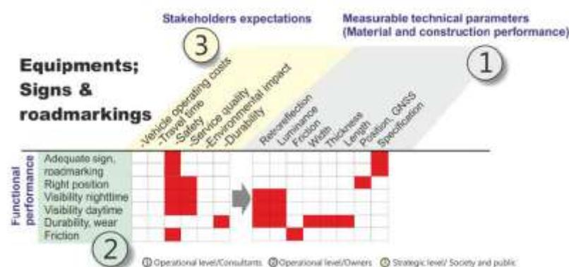
Figure 3.36: Equipment, signs and roadmarkings technical parameters
