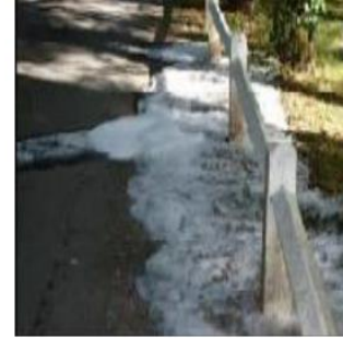
Figure 25: Hydro thermal weed cleaner with hot water foam system. Source (Ajuntament de Barcelona 2016)
