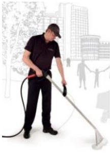
Figure 25: Hydro thermal weed cleaner with hot water foam system. Source (Ajuntament de Barcelona 2016)
