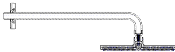
Figure 27: Diagram of the metal showerhead
