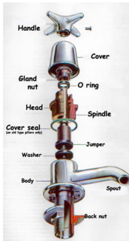
Figure 2 Components of a spindle tap
