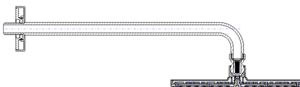
Figure 25: Diagram of the metal showerhead
