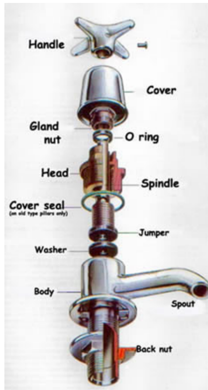
Figure 2 Components of a spindle tap
