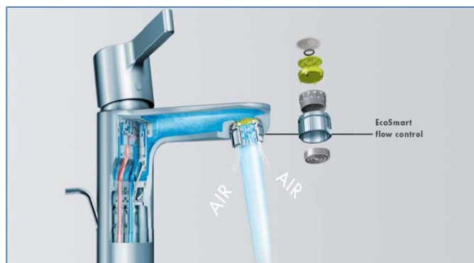
Figure 2: Example basin mixer (Metris S) fitted with an integrated aerator and flow regulator 2
