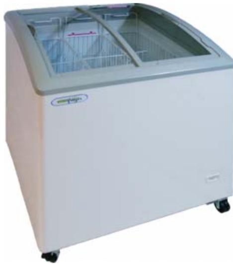
Figure 4 Packaged horizontal ice cream freezer with lids (category IHF6 according to EN ISO 23953), with a net volume of 291 litres, operating in temperature class L1 (-23°C to -18°C), using R507 as refrigerant, with a product life of 8 years. Plug-in.
