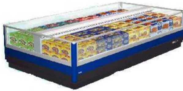
Figure 2 Open remote horizontal frozen island (category RHF4 according to EN ISO 23953), with 7 m 2 TDA, operating in temperature class L2 (-18°C to -12°C), using R404a as refrigerant, with a product life of 9 years.
