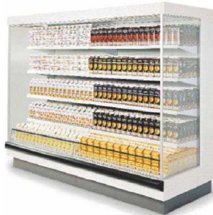
Figure 1 Open-chilled vertical multi-deck remote refrigerating display cabinet (category RVC2 according to EN ISO 23953), with 7 m 2 TDA, operating in temperature class M2 (-1°C to 7°C), using R404a as refrigerant, with a product life of 9 years.
