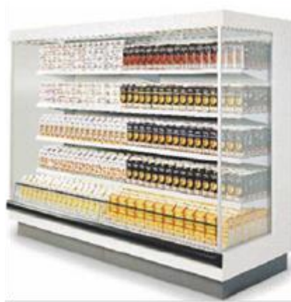
Figure 1 Open vertical multi-deck remote refrigerating display cabinet for chilled products (category RVC2 according to EN ISO 23953), with 7 m 2 TDA, operating in temperature class M2 (-1°C to 7°C), using R404a as refrigerant, with a product life of 9 years.
