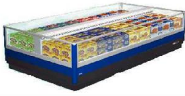
Figure 2 Open remote horizontal island for frozen products (category RHF4 according to EN ISO 23953), with 7 m 2 TDA, operating in temperature class L1 (-18°C to -15°C), using R404a as refrigerant, with a product life of 9 years.
