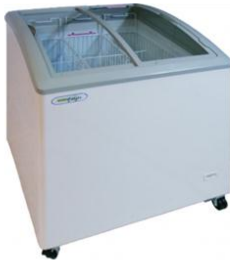
Figure 4 Packaged horizontal ice cream freezer with lids (category IHF6 according to EN ISO 23953), with a net volume of 291 litres, operating in temperature class L1 (-18°C to -15°C), using R507 as refrigerant, with a product life of 8 years. Plug-in.
