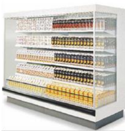
Figure 2-1 Open vertical multi-deck remote refrigerating display cabinet for chilled products (category RVC2 according to EN ISO 23953), with 7 m 2 TDA, operating in temperature class M2 (-1°C to 7°C), using R404a as refrigerant, with a product life of 9 years.
