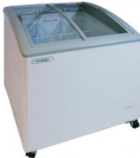
Figure 2-4 Packaged horizontal ice cream freezer with lids (category IHF6 according to EN ISO 23953), with a net volume of 291 litres, operating in temperature class L1 (-18°C to -15°C), using R507 as refrigerant, with a product life of 8 years. Plug-in.
