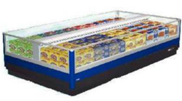
Figure 2-2 Open remote horizontal island for frozen products (category RHF4 according to EN ISO 23953), with 7 m 2 TDA, operating in temperature class L1 (-18°C to -15°C), using R404a as refrigerant, with a product life of 9 years.
