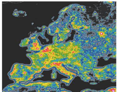
Even if light levels do not increase in terms of lumens on the road, replacing HPS lights with LED could result in a significant increase in sky brightness.
