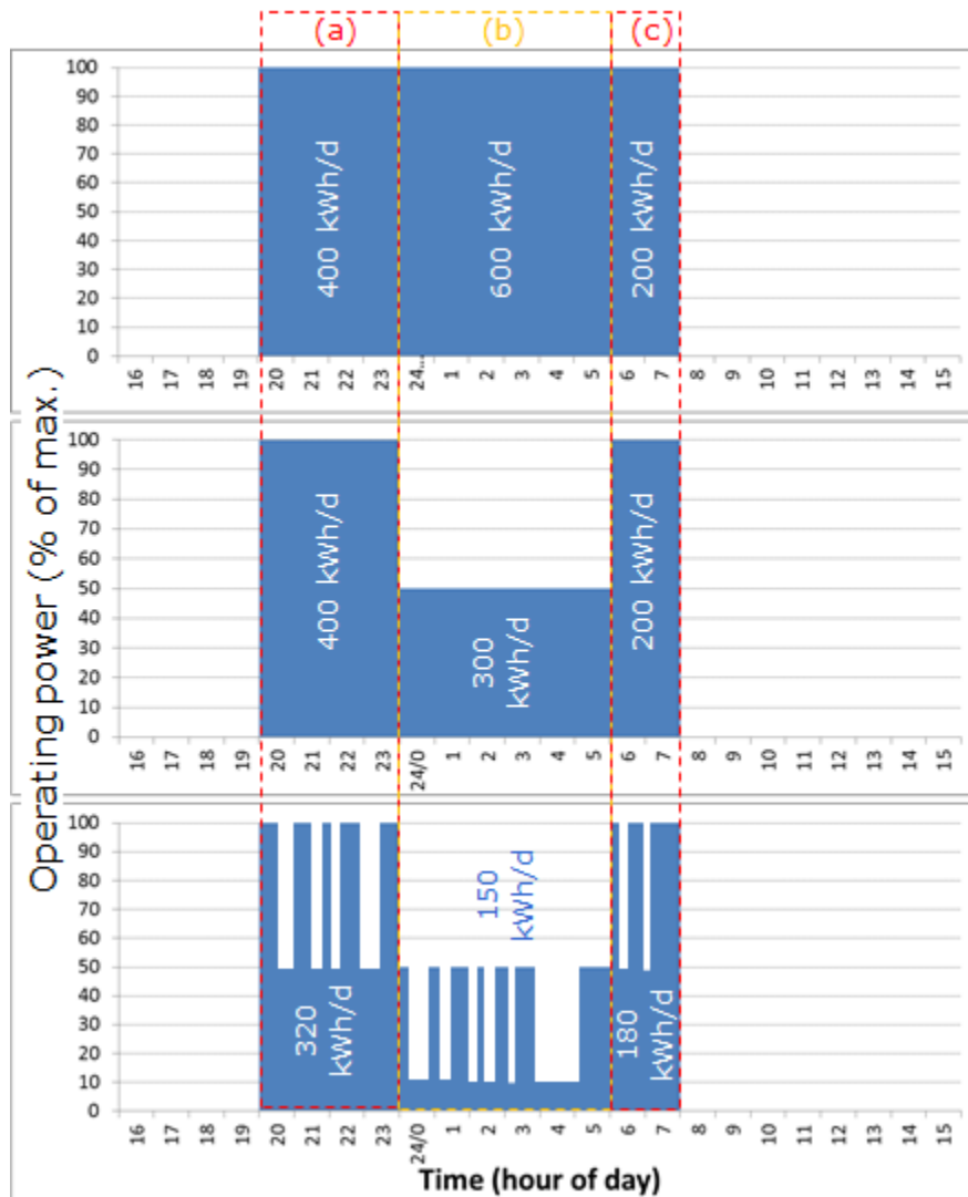
Figure 11. Examples of different operational profiles for road lighting installations during period a) evening peak hours, b) off-peak hours and c) morning peak hours (adapted from EN 13201-5). Consumption figures included refer to a 100kW installation
