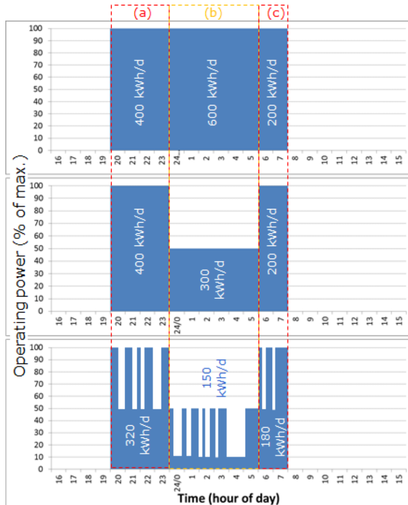
Figure 14. Examples of different operational profiles for road lighting installations during period a) evening peak hours, b) off-peak hours and c) morning peak hours (adapted from EN 13201-5). Consumption figures included refer to a 100kW installation
