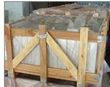
loose gaps tightened with filling material like wood, foamsheet
