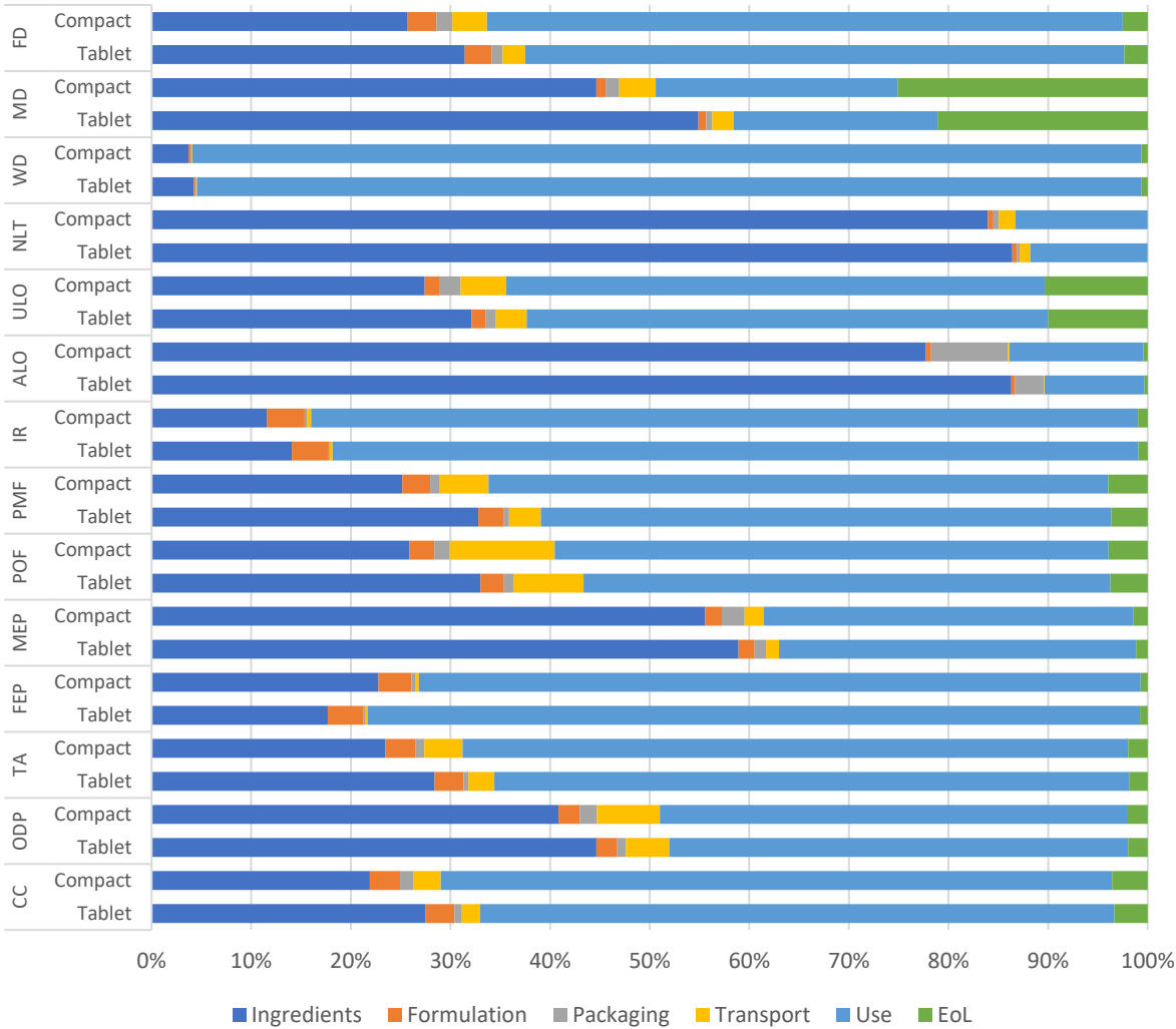
Figure 55. Comparison of relative midpoint impacts for compact powder format and tablet format laundry detergents. Source: Golsteijn et al., 2015.
