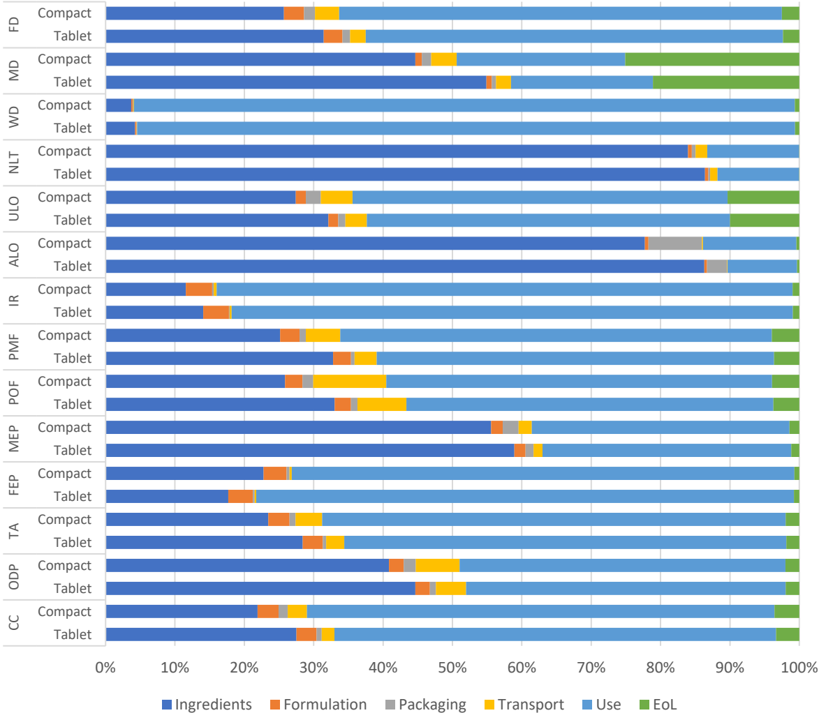
Figure 48. Comparison of relative midpoint impacts for compact powder format and tablet format laundry detergents. Source: Golsteijn et al., 2015.
