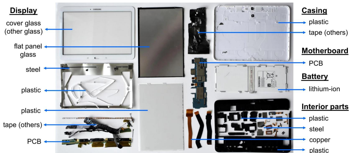
Figure 5: Example of product disassembly for a tablet (Samsung Galaxy Tab 4 SM-T530, 2014), illustrating the main components (Babbitt et al., 2020).
