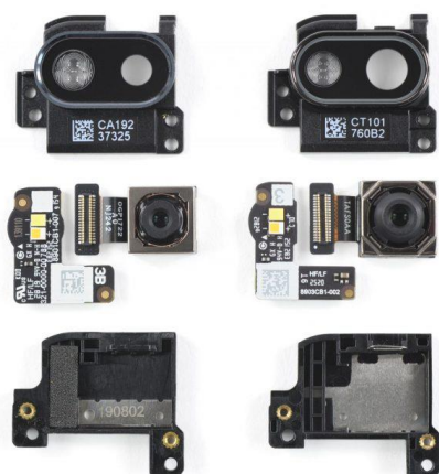
Figure 36: modular components of the Fairphone 3 smartphone.
