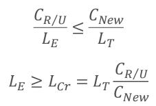
Illustration of the relationship between failure time and expected future lifetime.
