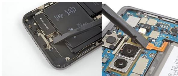
Figure 15. Example of connector's disconnection in 2 different models of smartphone. [Source: iFixit.com]
