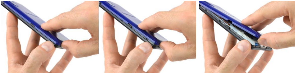
Figure 18. Example of back cover with a “reusable” snap-fit fastening system and replaceable with “no tools” [Source: iFixit.com]
