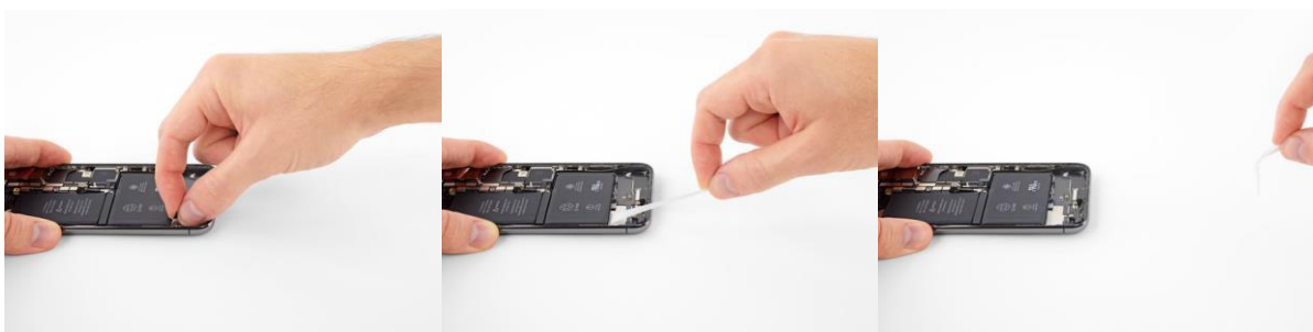
Figure 17. Example of “removable” pull-tab adhesive [Source: iFixit.com]
