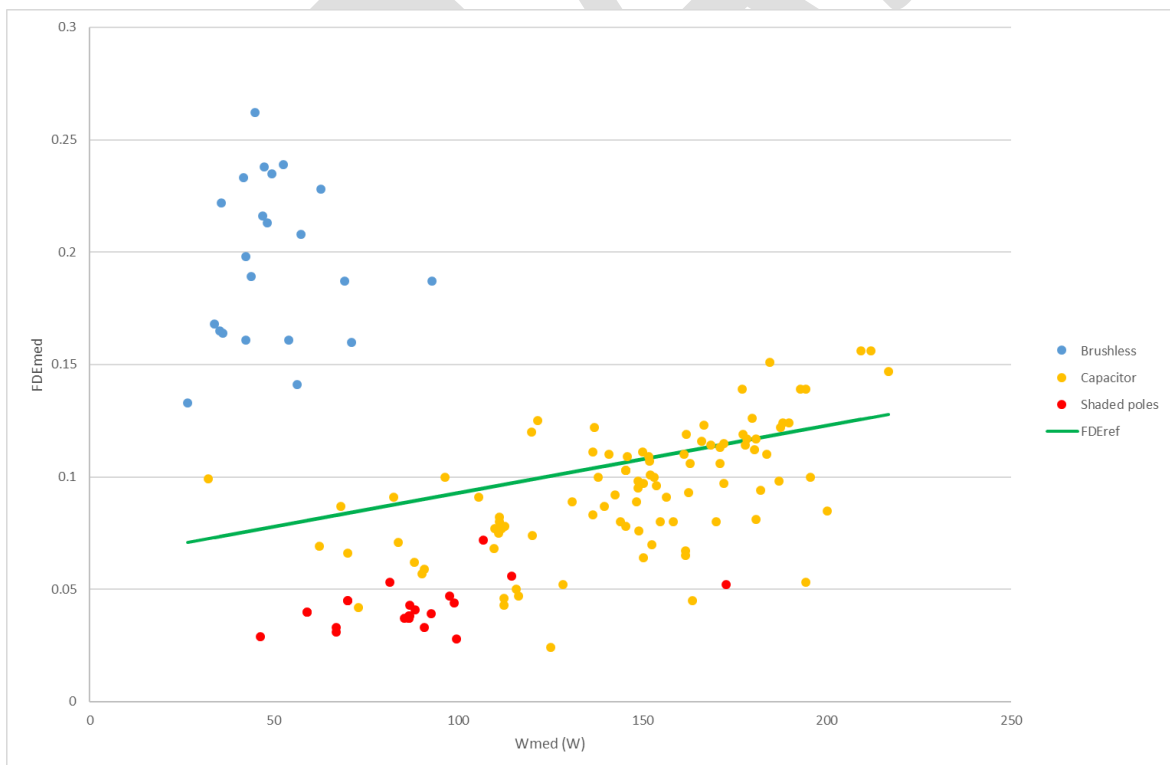
Figure 305: FDE, FDEref and power calculated as 9-points average
