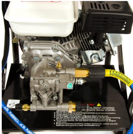
NB: An example of a combustion engine, where the pump is driven directly by the main shaft of the engine. In some configurations the pump may be driven indirectly via a belt.
