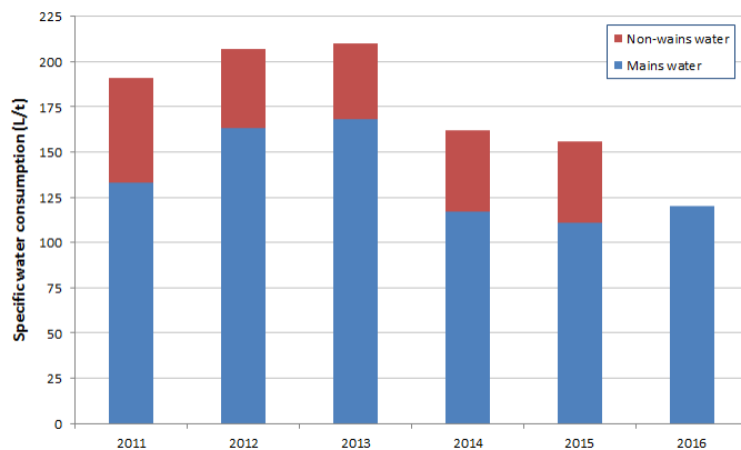
Figure 30. Trend in specific water consumption for the UK brick industry.
