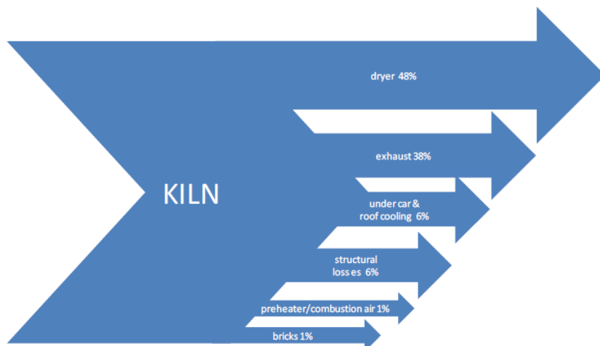
Figure 23. Sankey diagram for fuel energy flows from the kiln in brick production (Source: Carbon Trust, 2010)
