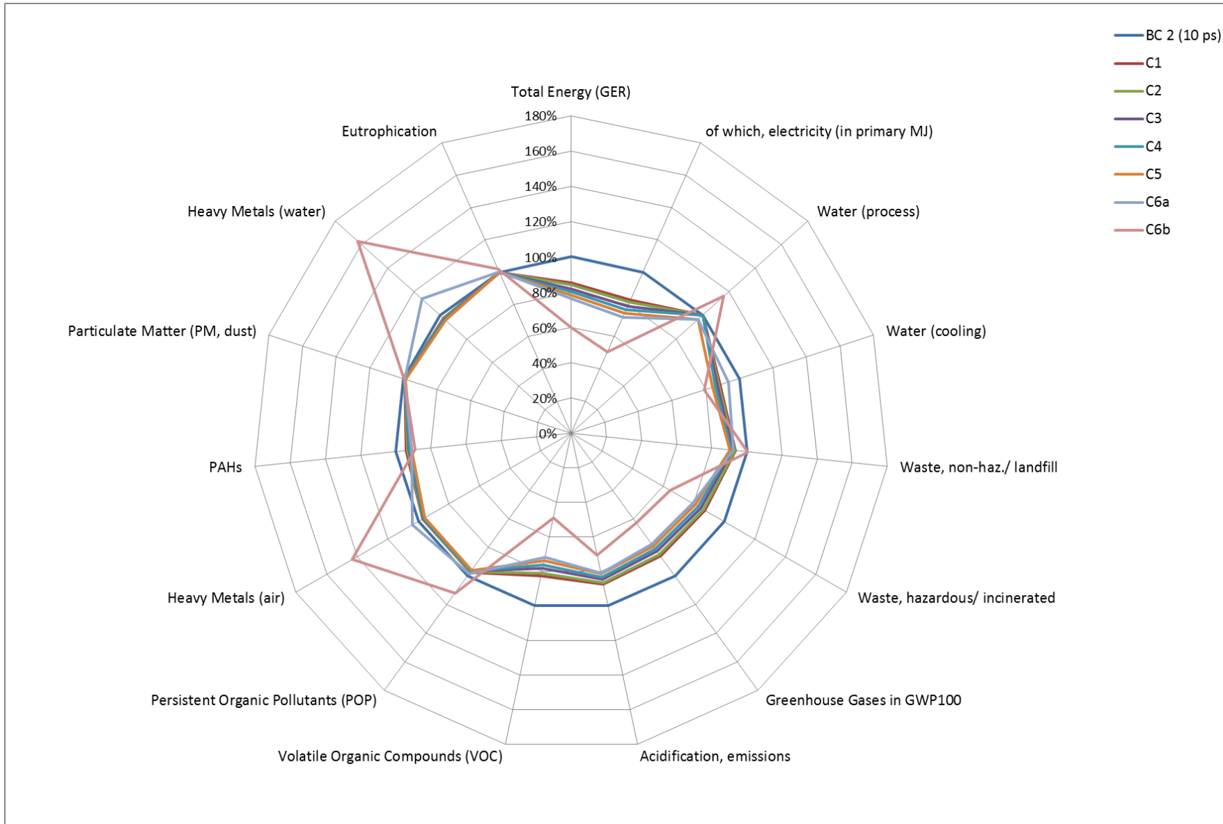
Figure 6-4: Relative environmental impacts of the combinations of design options compared to the slim-line Base Case 2 (10 ps)
